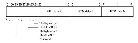
Figure 11-6 Integration ETM Data bit assignments
