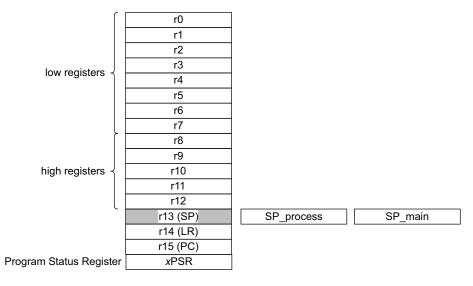
Figure 3-3 Processor register set
