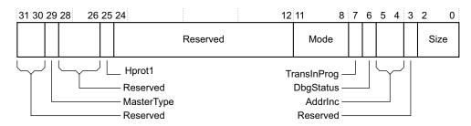
Figure 8-2 CSW bit assignments
