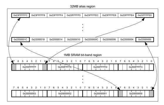
Figure 3-2 Bit-band mapping
