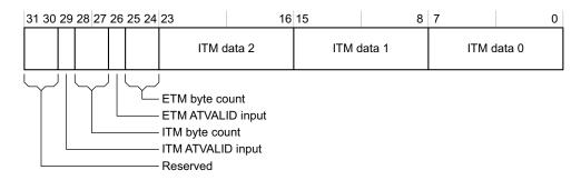
Figure 11-8 Integration ITM Data bit assignments
