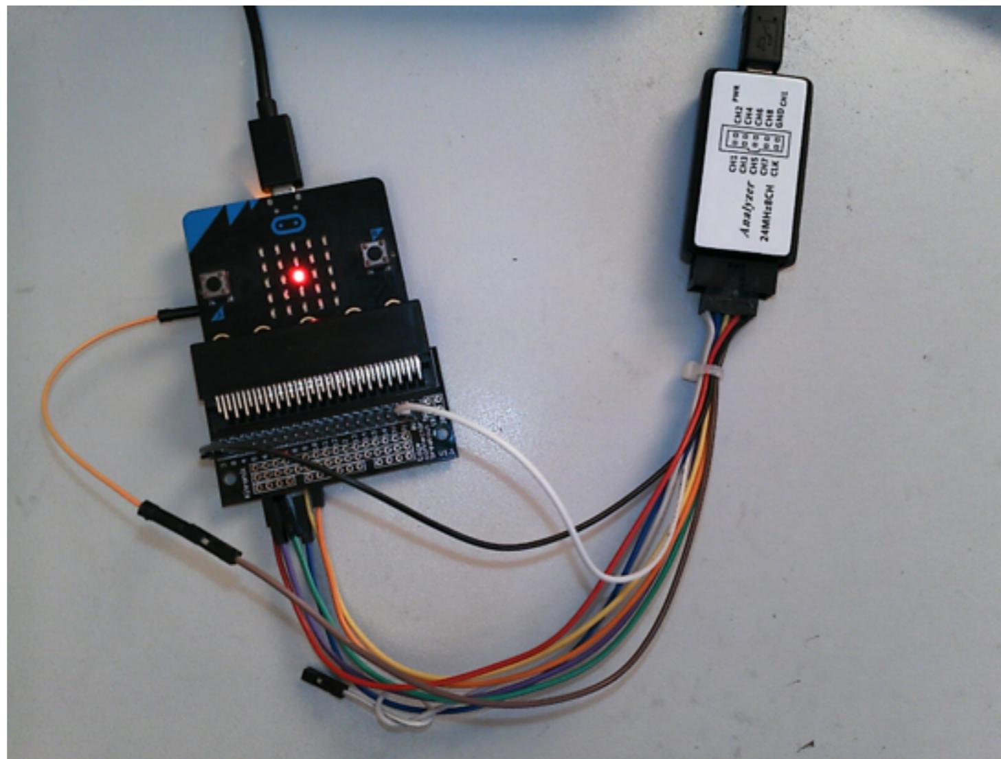
Monitoring both an LED pin and the UART
