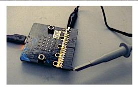
Ground clip to ground Probe to an LED pin
